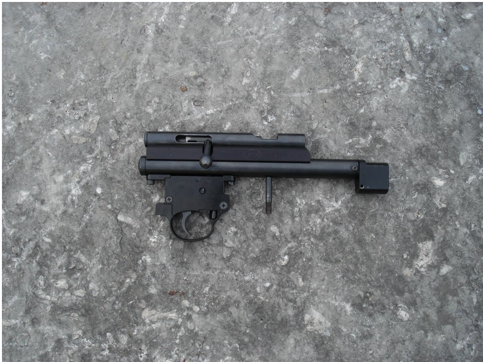
Qb79 action with spacer installed
